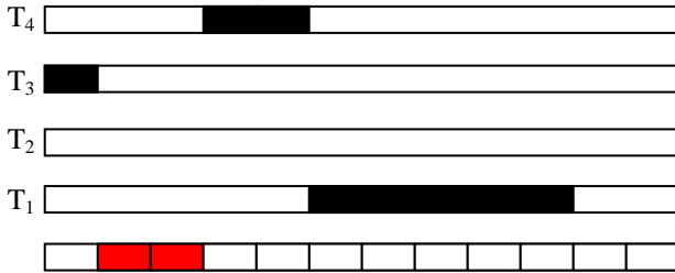
Fig. 2. Gantt chart of scheduled tasks with ADAF in case of transient timing fault on single processor system.
